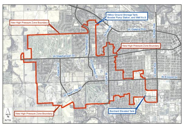
Although much of the City will not be in the new pressure zone, the isolation of this area will change how water travels throughout the majority of the City. In many cases, water will reverse flow from how it has traveled for decades, causing iron buildup within our pipe network to break free. The increases in pressure to older pipes within the new pressure zone may also contribute to additional water main breaks.
